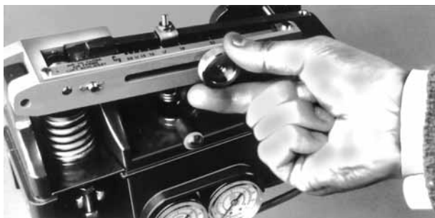
Figure 4 - Adjusting the C_v of VariPak 28002 valve for each plug/seat ring combination
